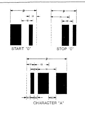
Figure 7 Decode Measurements
