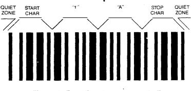
Figure 1. Encoding the message "1A"
