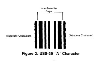
Each bar or space can be one of two alternative widths, referred to as "wide" and "narrow". The particular pattern of wide and narrow bars determines the character being coded. In all cases, each character consists of three wide and six narrow elements.
