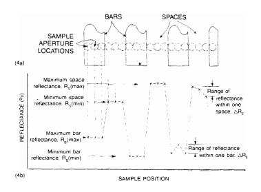
Figure 4. Bar Code Reflectance Measurements
