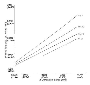
Figure 3 USS-39 Dimensional Tolerances
