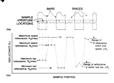
Figure 5. Bar Code Reflectance Measurements
